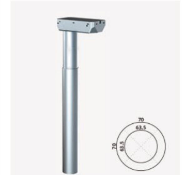
Model: DL10 Stroke Length: 500mm Lowest Position: 650mm Highest Position: 1150mm Load Capacity :800N Speed: 28-36mm/s
