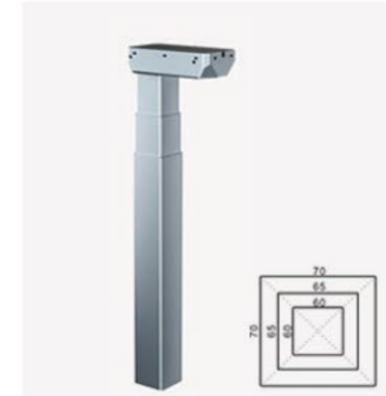
Model: DL19 Stroke Length: 650mm Lowest Position: 560mm Highest Position: 1210mm Load Capacity :800N Speed: 35mm/s
