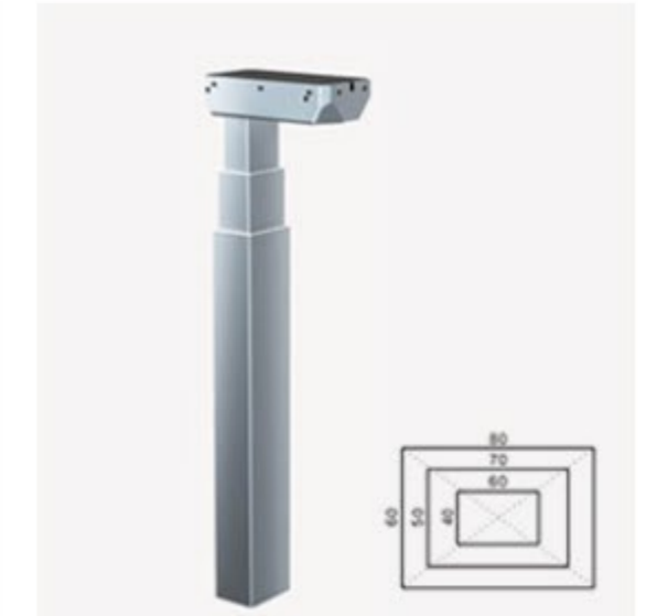
Model: TL10 Stroke Length: 650mm Lowest Position: 560mm Highest Position: 1210mm Load Capacity :800N Speed: 35mm/s
