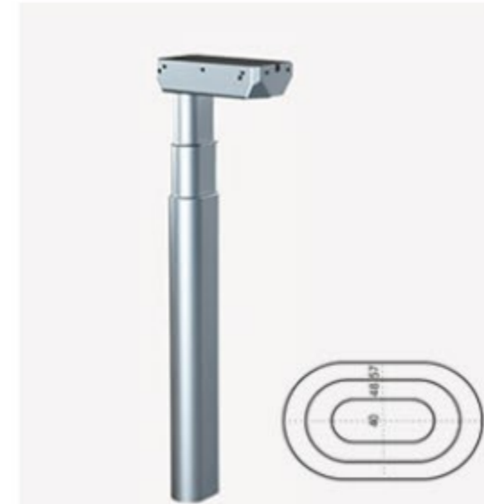
Model: DL4 Stroke Length: 650mm Lowest Position: 560mm Highest Position: 1210mm Load Capacity :800N Speed: 35mm/s
