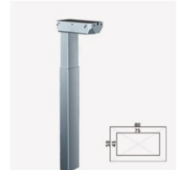
Model: DL5 Stroke Length: 500mm Lowest Position: 650mm Highest Position: 1150mm Load Capacity :800N Speed: 28-36mm/s
