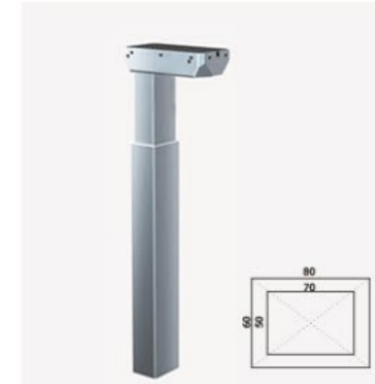
Model: TL10 Stroke Length: 500mm Lowest Position: 650mm Highest Position: 1150mm Load Capacity :800N Speed: 28-36mm/s
